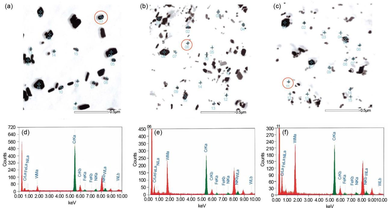
**Figure 8.** Scanning transmission electron images ((a) virgin (b) pre-strained at 10% (c) pre-strained at 15%) and results of EDX analysis taken from the precipitates in grains of HR6W ((d) virgin (e) pre-strained at 10% (f) pre-strained at 15%).
