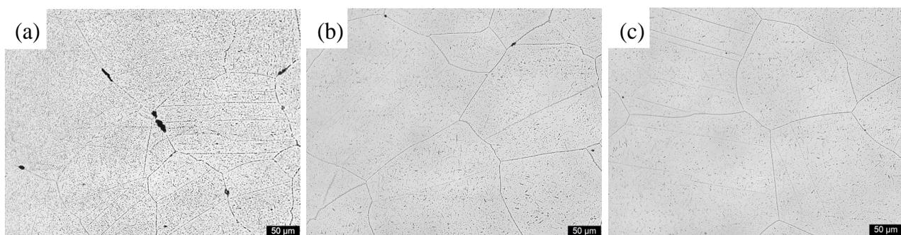
**Figure 3.** OM images of HR6W ruptured at 750°C, 90 MPa for 11,010 h ((a) virgin) and interrupted at 750°C, 100 MPa for 10,400 h ((b) pre-strained at 10% (c) pre-strained at 15%).
