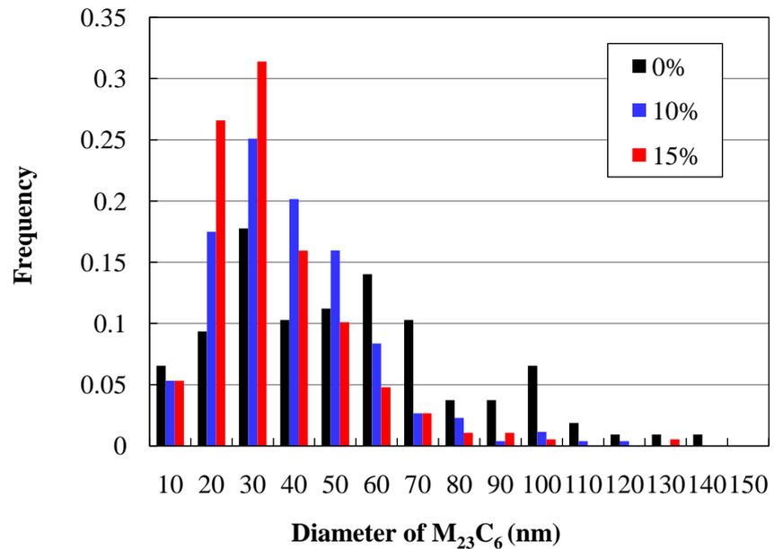
**Figure 9.** Histograms showing the distribution of diameters of  $\text{M}_{23}\text{C}_6$  carbide in HR6W with and without pre-strain.
