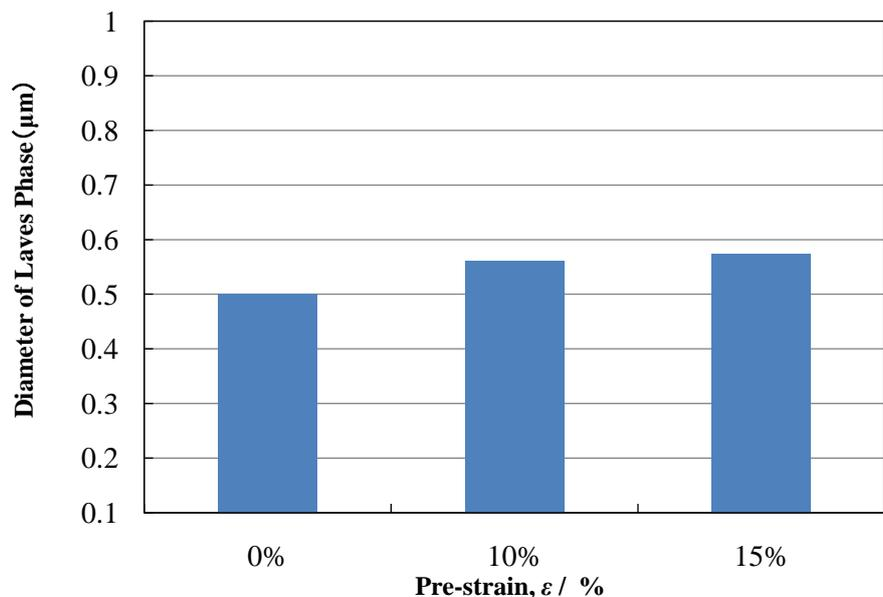
**Figure 7.** The average diameters of Laves phase for HR6W in virgin alloy after creep ruptured at 750°C, 90 MPa for 11,010 h and pre-strained alloy after creep interrupted at 750°C, 100 MPa for 10,400 h.
