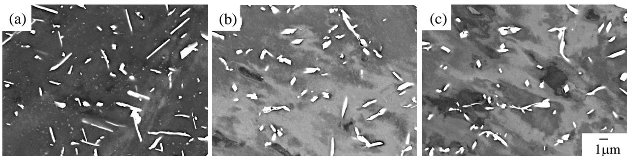
**Figure 6.** Backscattered electron images of intragranular grain for HR6W ruptured at 750°C, 90 MPa for 11,010 h ((a) virgin) and interrupted at 750°C, 100 MPa for 10,400 h ((b) pre-strain at 10% (c) pre-strain at 15%).
