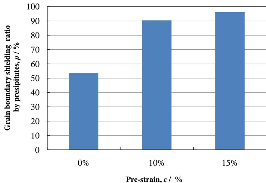
**Figure 5.** The ratio of grain boundary shielding by precipitates in HR6W crept at 750°C for 11,010 h without pre-strain and at 750°C for 10,400 h with pre-strain.
