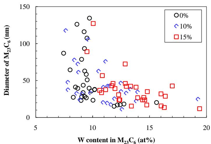
Figure 11. The relationship between W content in  $M_{23}C_6$  carbide and its diameter.
