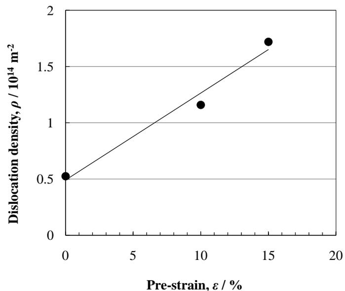
**Figure 10.** Change in the dislocation density with the amount of pre-strain in HR6W.
