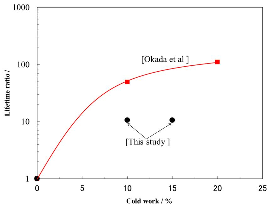
**Figure 2.** The effect of pre-strain on the creep rupture time of HR6W.
