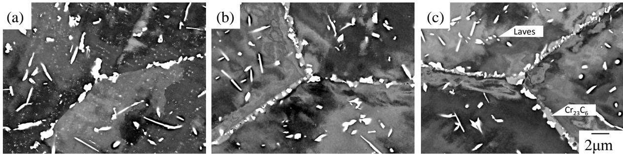
**Figure 4.** Backscattered electron images of grain boundaries for HR6W ruptured at 750°C, 90 MPa for 11,010 h ((a) virgin) and interrupted at 750°C, 100 MPa for 10,400 h ((b) pre-strained at 10% (c) pre-strained at 15%).
