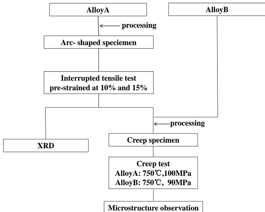
**Figure 1.** Flow diagram of experimental procedure.
