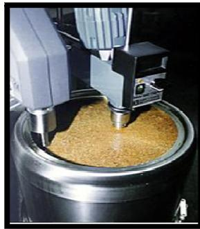
**Fig. 1(b). Ultrasonic Extraction (Hielscher, USA) (University of Nottingham Malaysia)**
