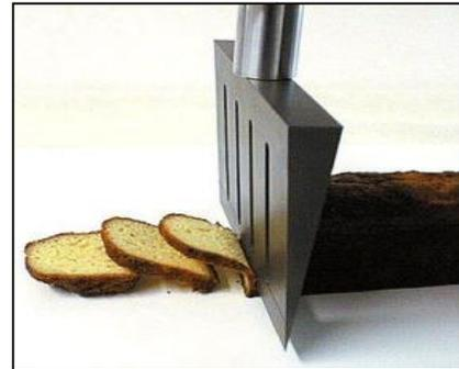
**Fig. 1(c). Ultrasonic Cutting (Hangzhou Altrasonic Technology Co., Ltd, China)**
